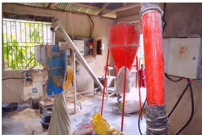
BICODA's mill processing maize into flour
